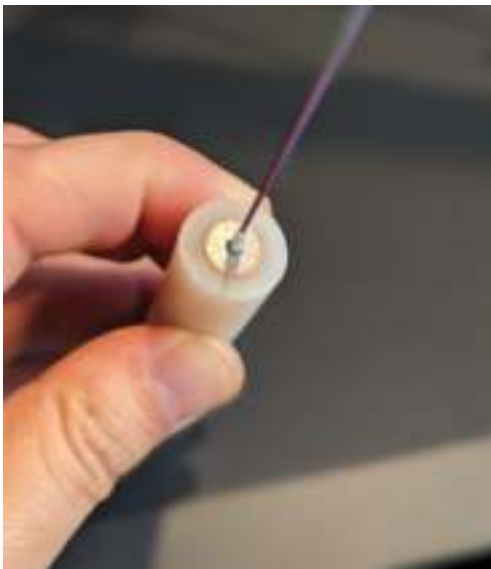
“Lightweight” core cable Used in deep water About ½ inch diameter
